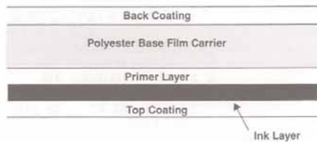
Figure 3 - Thermal Transfer Ribbon Construction
